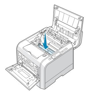
**12** To replace the transfer belt, hold its handle and then align it with the slots inside your printer, on each side.
